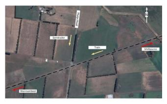
This sighting issue is exacerbated by the acute angle between the road and rail geometry, which present further challenges for road users to identify an oncoming train. It is noted in the collision report that the angle is non-compliant with level crossing design standards.
